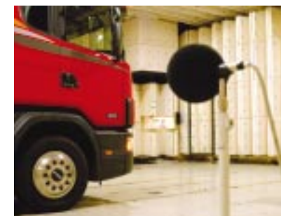
External noise levels are measured both by means of laboratory experiments and field tests.
