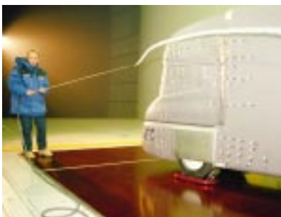
New aerodynamic solutions are mainly tested by means of wind tunnel experiments.
